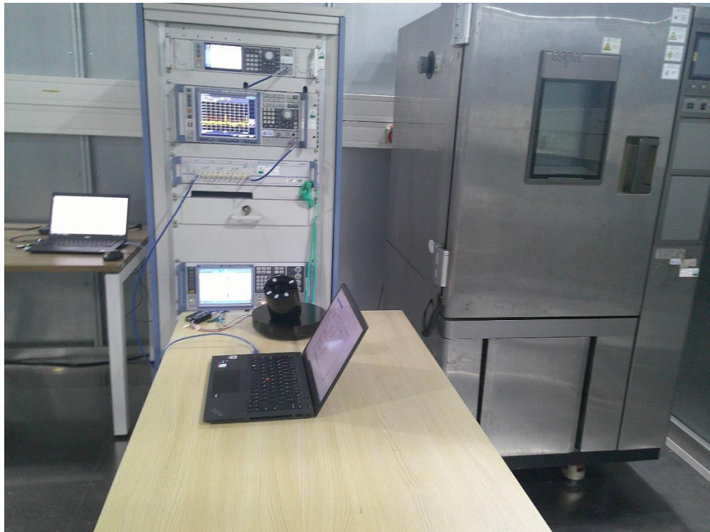
Photograph 1: Set-up photo for RF Conducted Test
