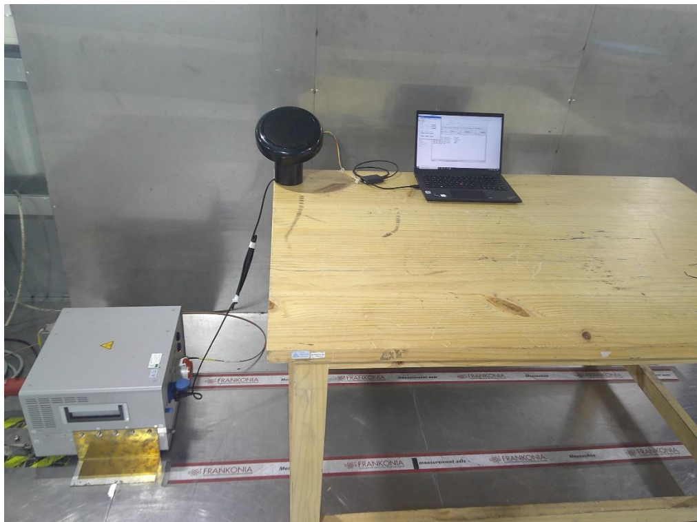
Photograph 2: Set-up photo for Conducted Emission
