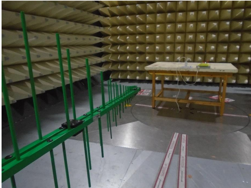
Photograph 3: Set-up for measurement of radiated emission
