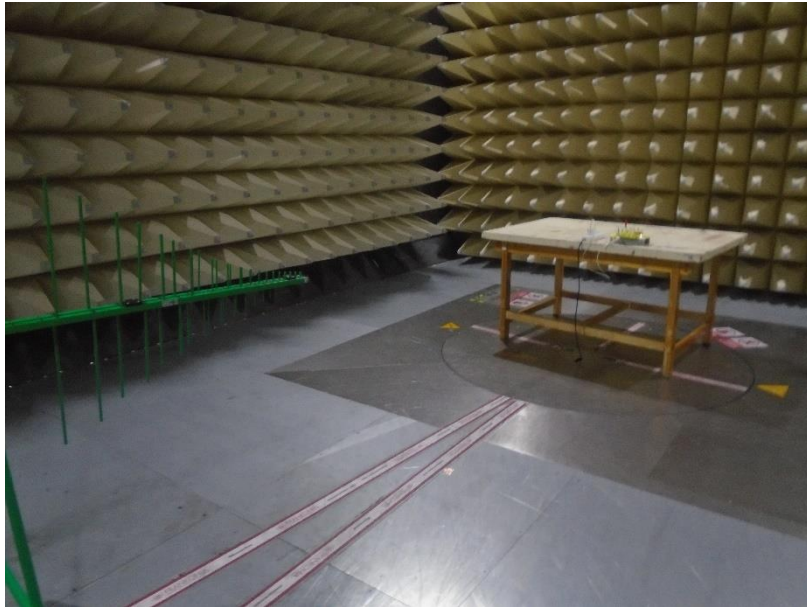
Photograph 3: Set-up for measurement of radiated emission
