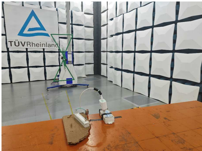
Photograph 2: Set-up for measurement of radiated emission
