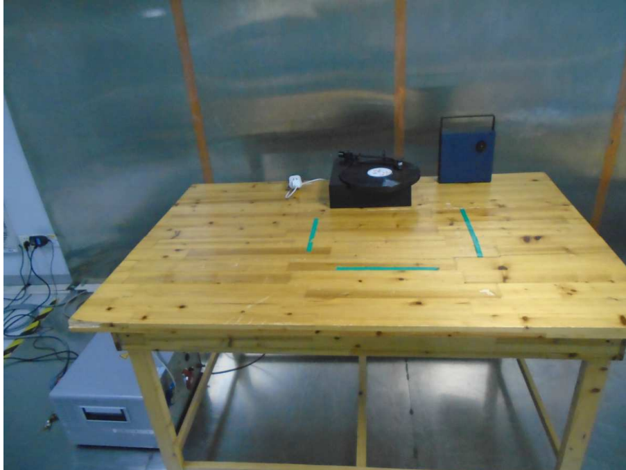
Photograph 1: Set-up for measurement of conducted emission
