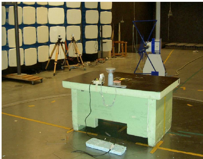
Test setup for conducted emission 150 kHz – 30 MHz
