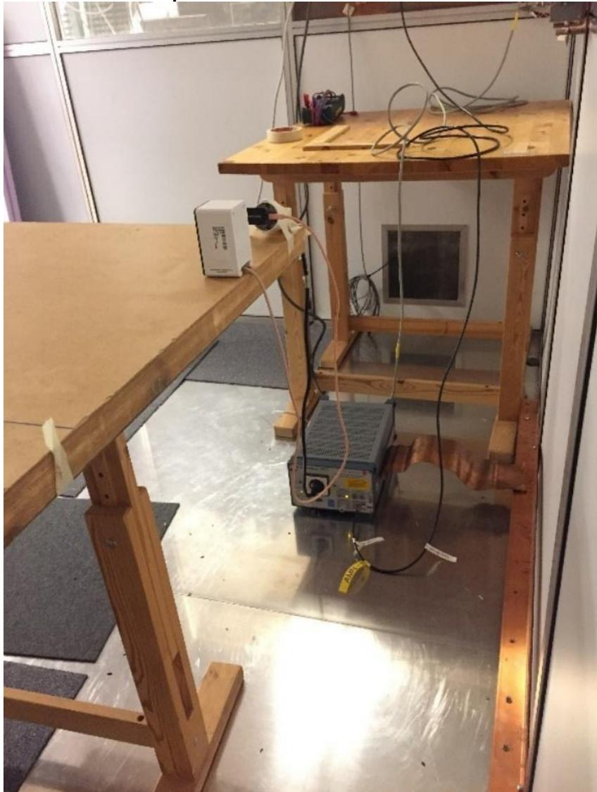
**Photo(s) of test setup(s) for conducted continuous disturbances**
