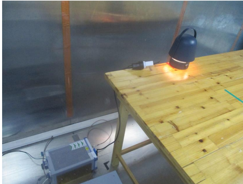
Photograph 2: Set-up for measurement of radiated emission
