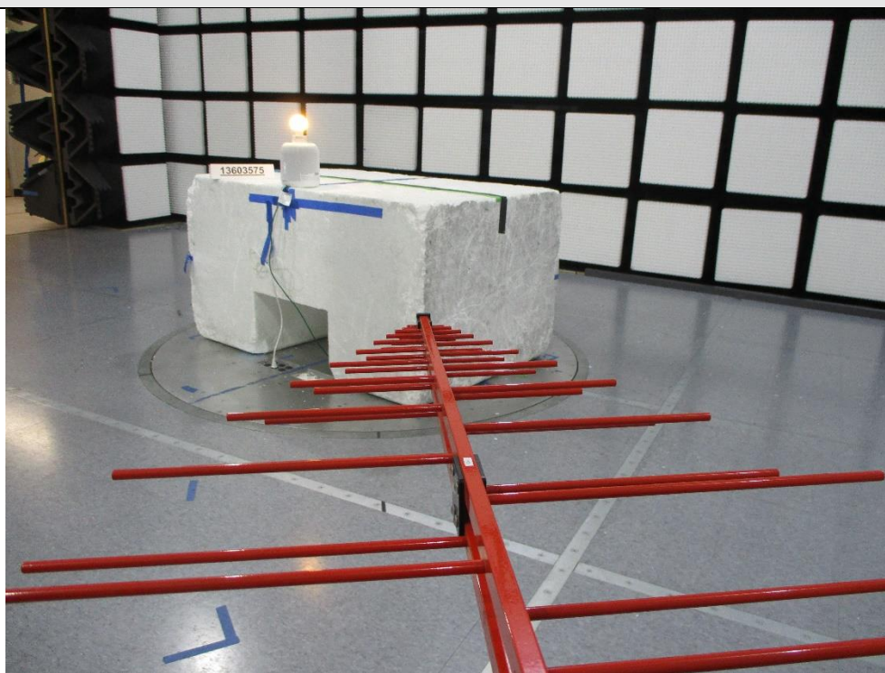
Photo of test setup for Radiated Emissions: 30-1000 MHz
