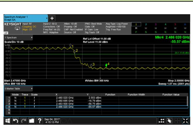
**DH5 Operation Frequency Range of 20dB Bandwidth within Hopping Mode**
