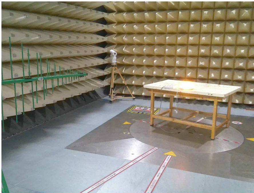
Photograph 2: Set-up for measurement of radiated emission
