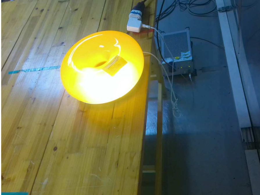
Photograph 1: Set-up for measurement of conducted emission
