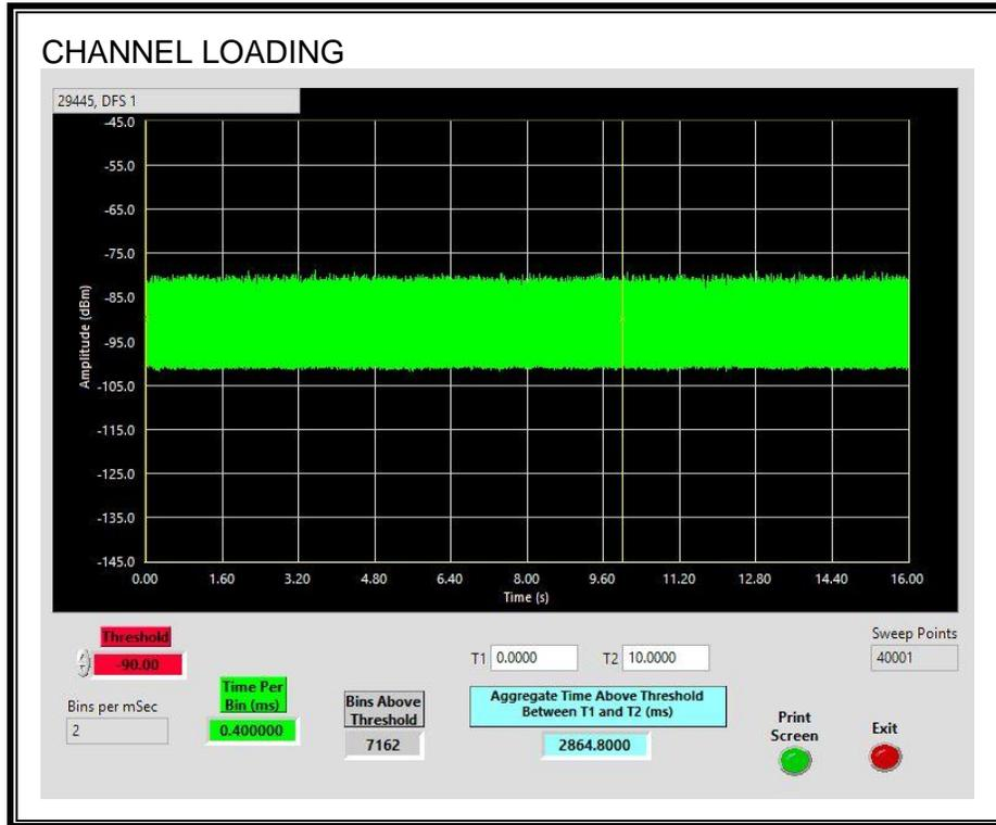
The level of traffic loading on the channel by the EUT is 28.64%
