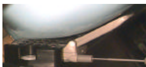
Figure 14. Head SAR Test Setup
