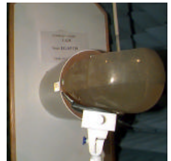
Figure 1. SAR Test Set-up
