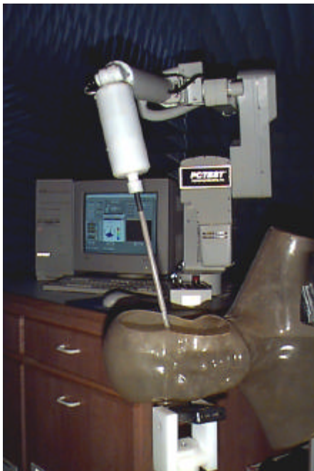
Figure 5. Photograph of the Probe and the Phantom
