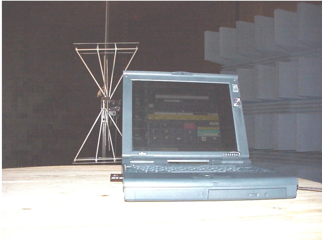
Test set up for radiated emissions:
