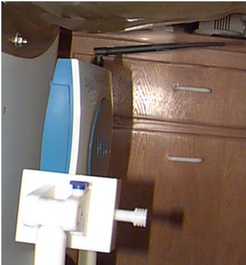
Figure 8. Test setup of EUT in normal operating position with the source of significant emissions (antenna) 2.0cm below the phantom.
