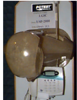
Figure 1. SAR Test Set-up
