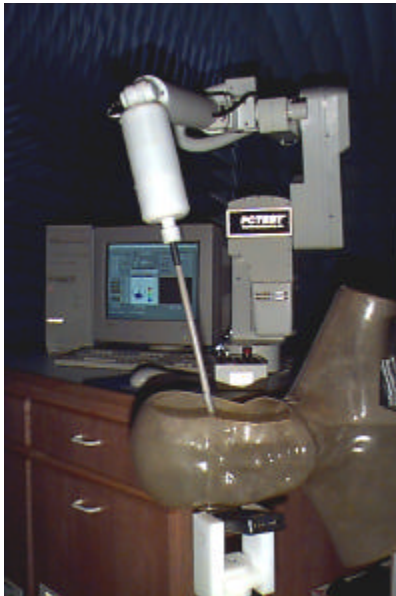
Figure 5. Photograph of the Probe and the Phantom
