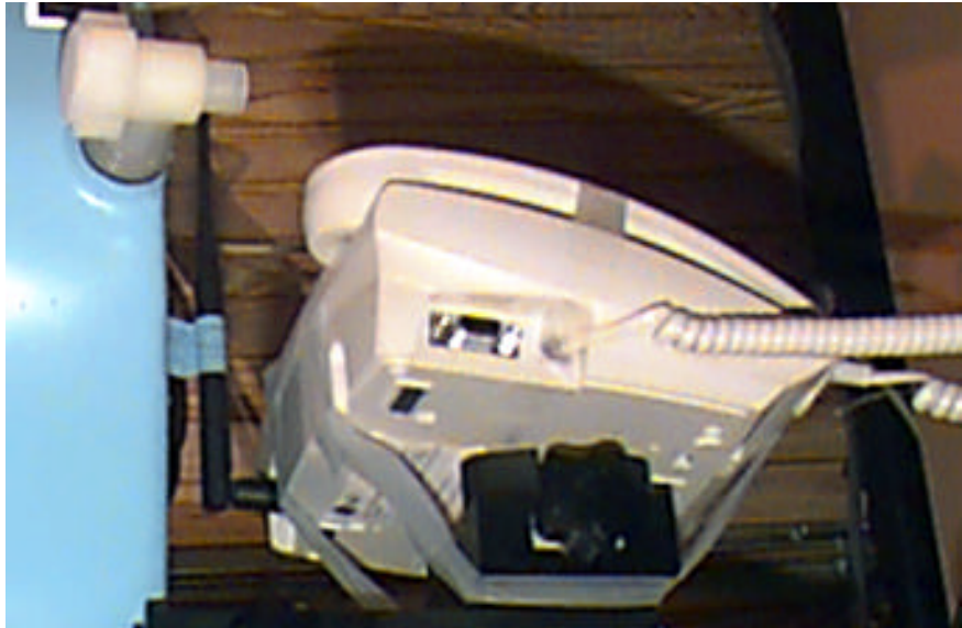
Figure 8. Actual placement of EUT with source of significant emissions placed 2 cm. from phantom surface.
