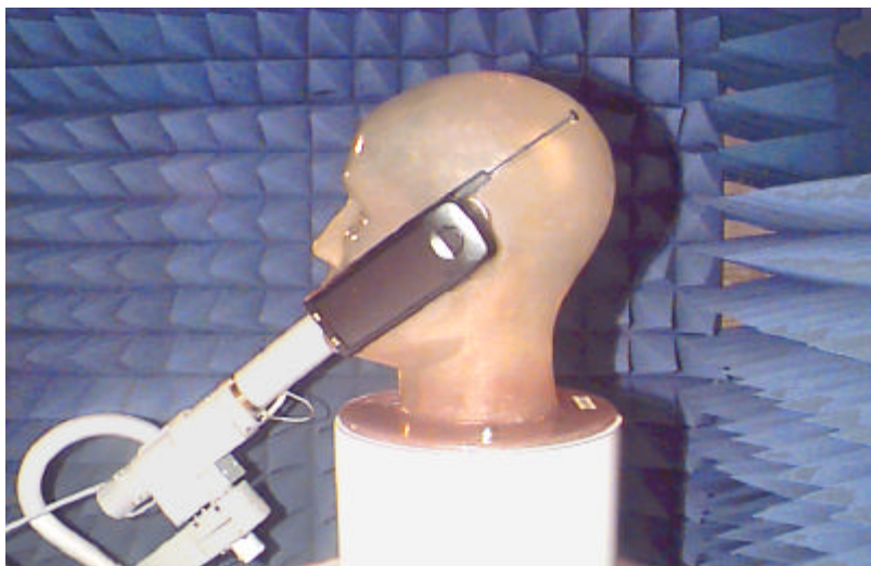
Figure 9. Sample of Handset alignment with the Ear Canal of the Phantom
