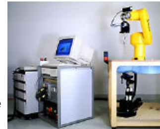
Fig. 1 SAR Test Setup
