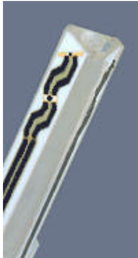
Fig. 5. ET3DV5 E-field Probe
