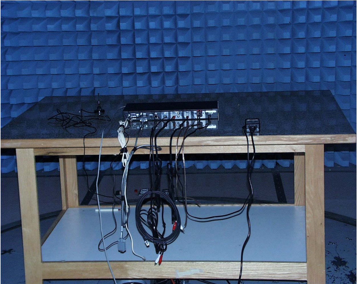
Back view of the Radiated Emissions Test Setup
