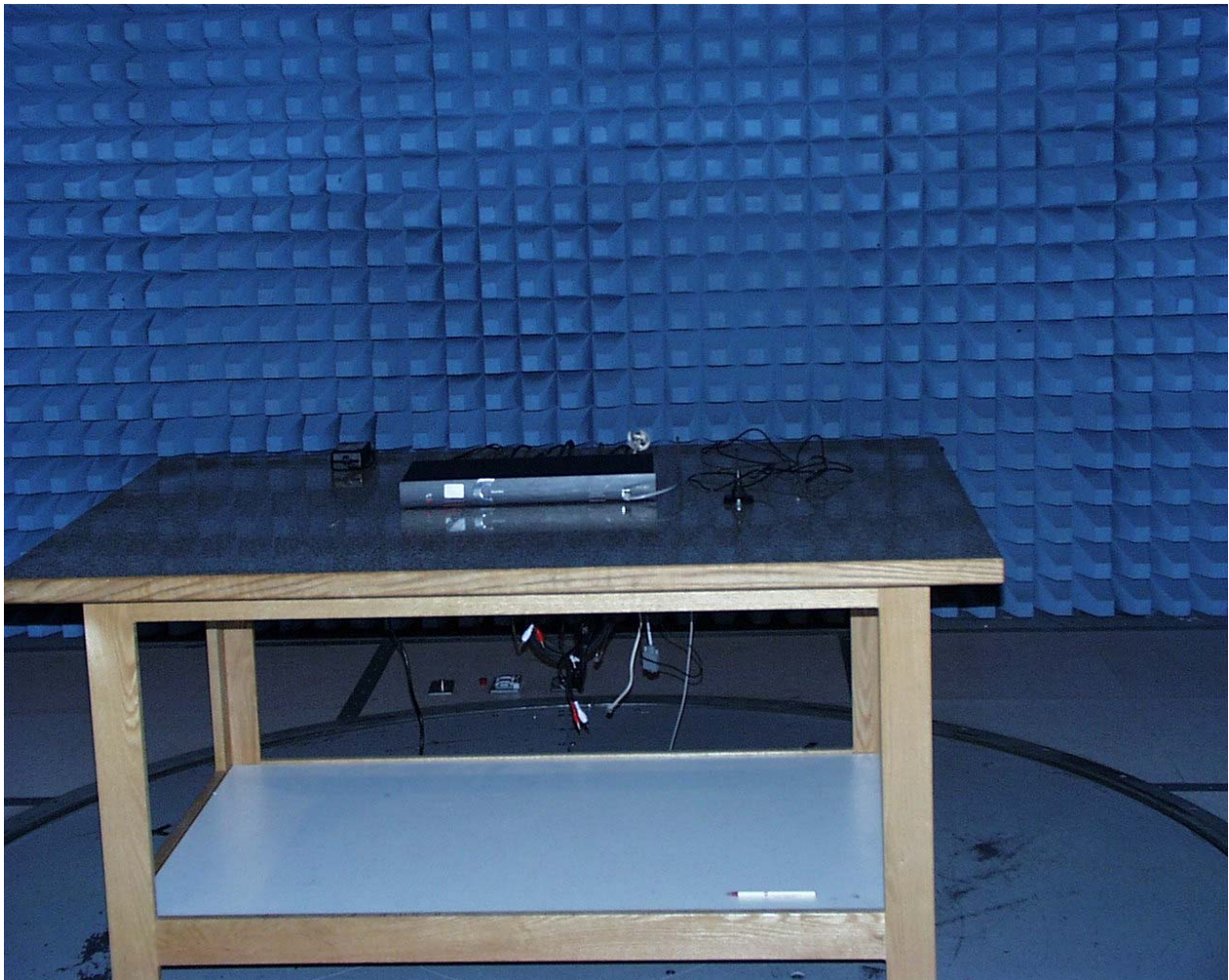
Front view of the Radiated Emissions Test Setup
