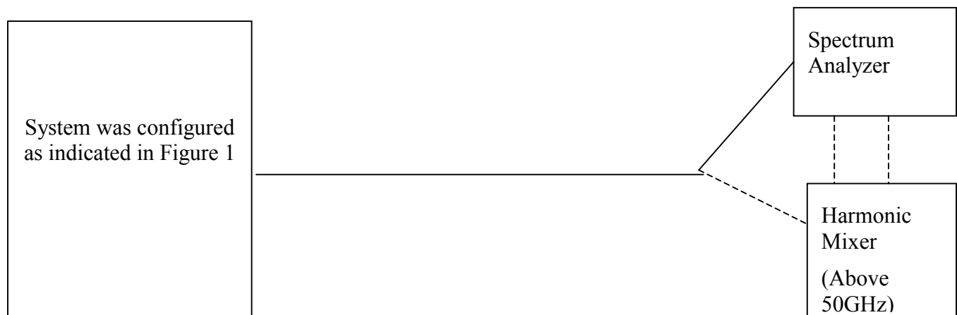
Figure – 5 Conducted Spurious measurement setup
