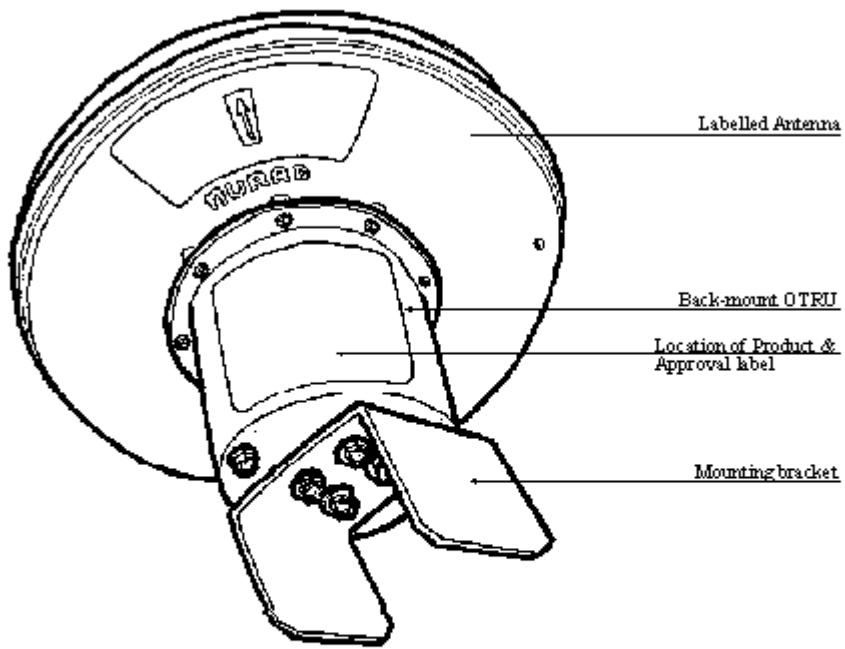
Applying "Product & Approvals Label" to Integrated Transceiver-Antenna Unit
