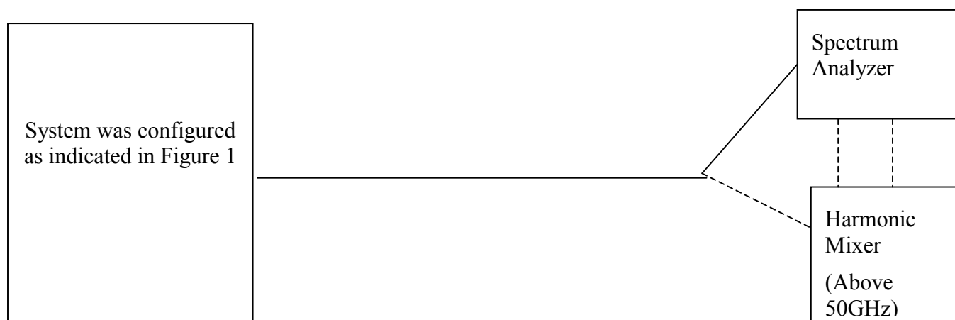
Figure – 5 Conducted Spurious measurement setup
