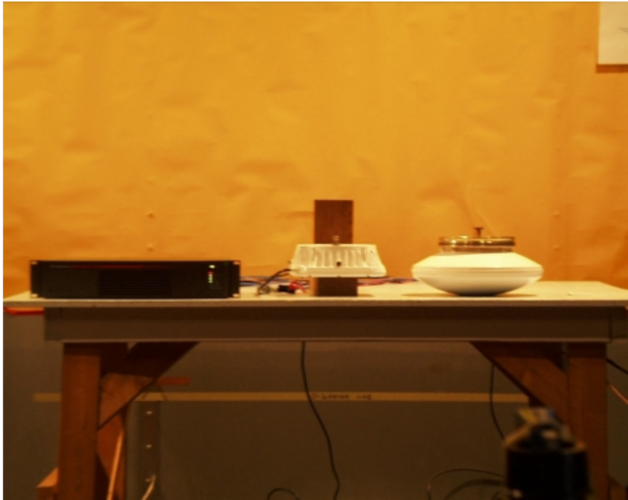
Radiated Spurious Setup in a Semi- Anechoic Chamber at KTL Ottawa Laboratories with OTRU terminated
