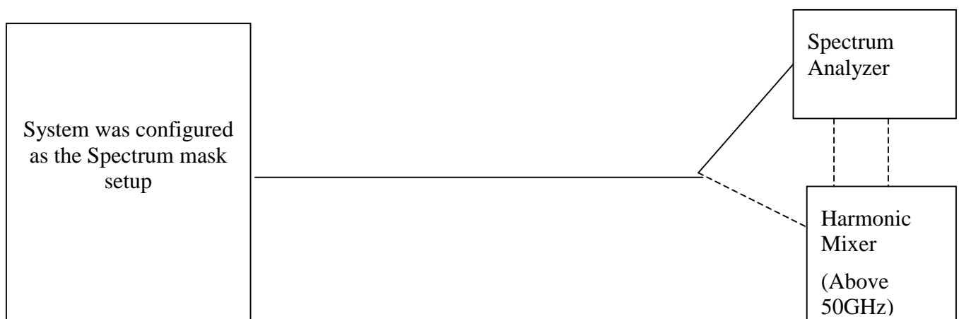
Conducted Spurious measurement setup
