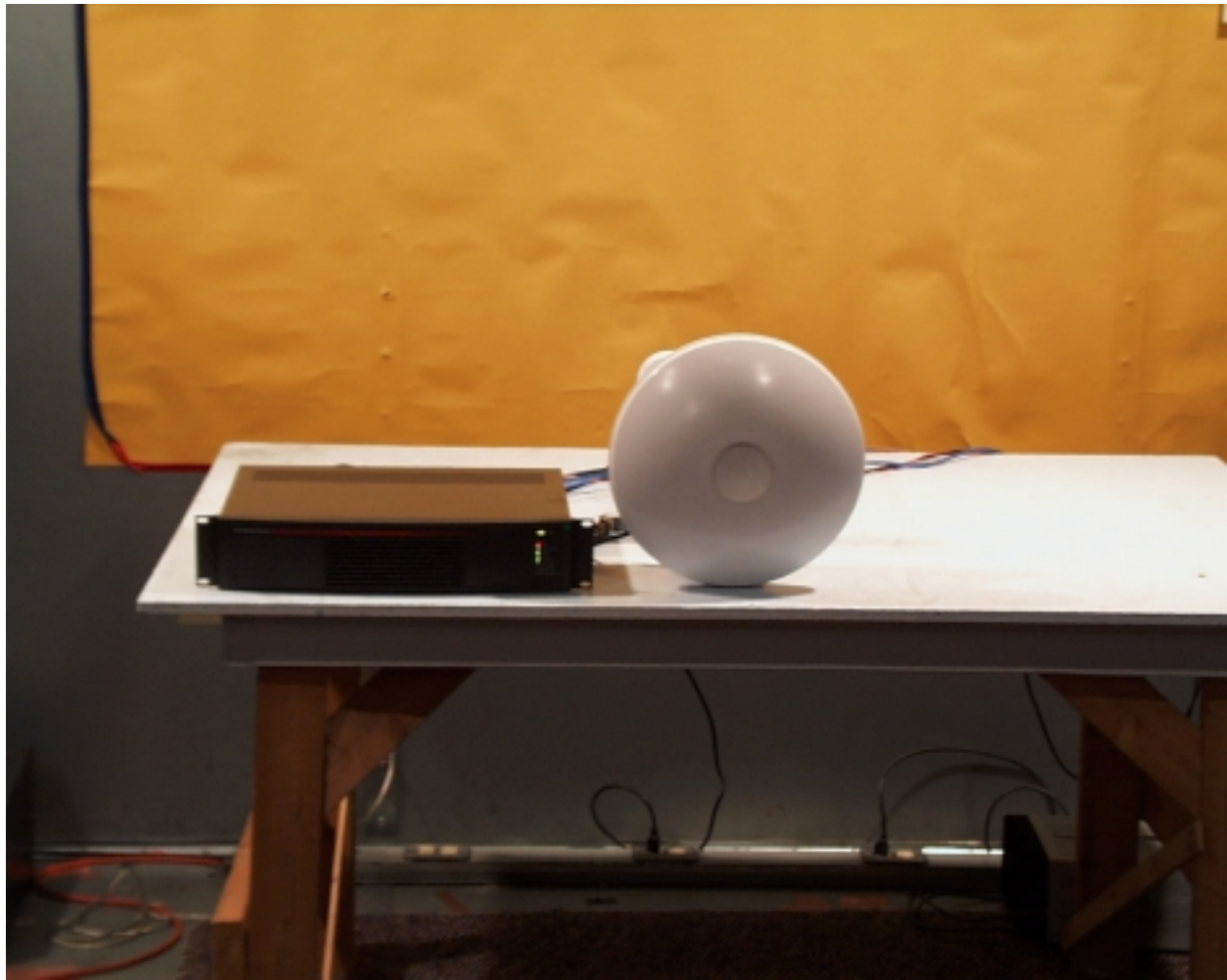
Radiated Spurious Setup front view in a Semi- Anechoic Chamber at KTL Ottawa Laboratories
