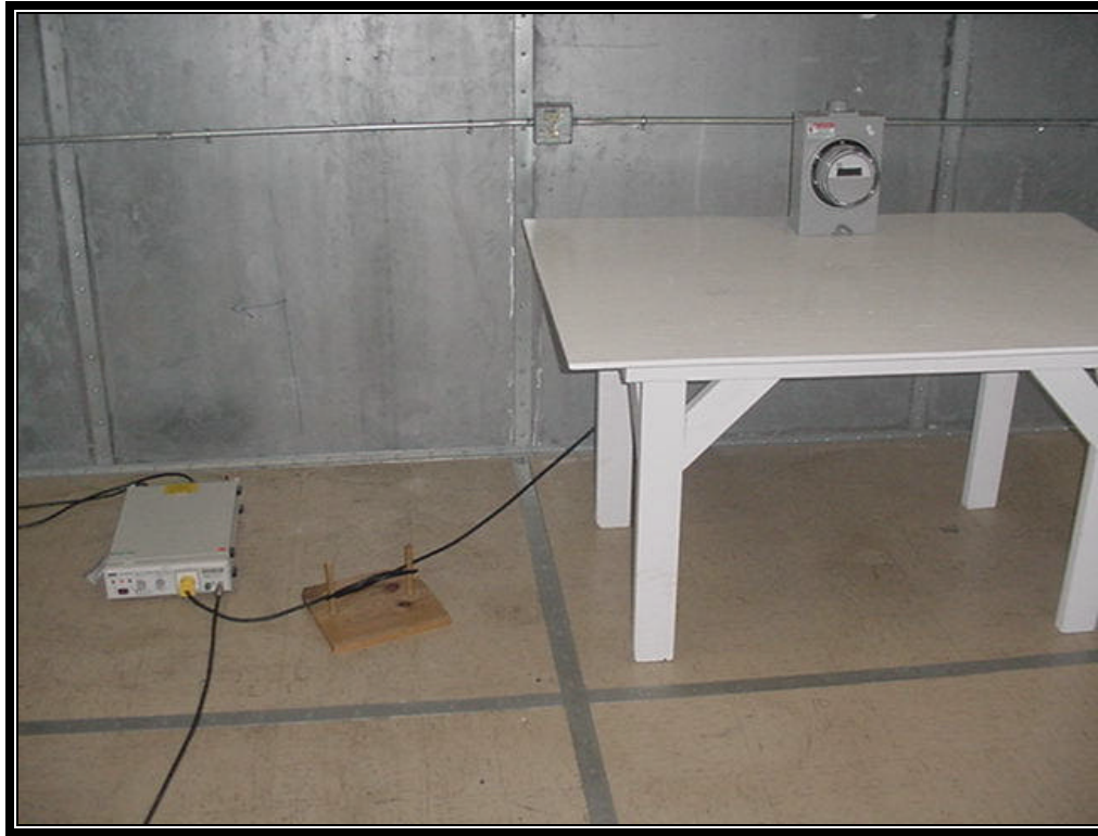
Figure 7.2-1: Conducted Emissions Test Setup
