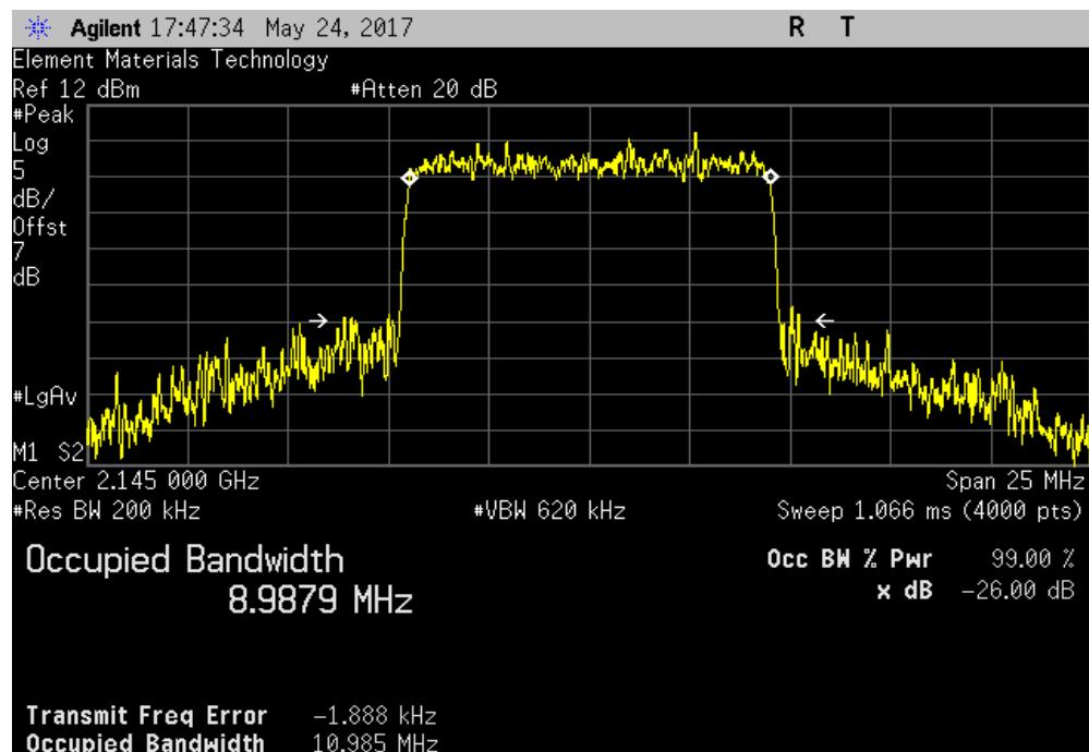
High Channel (2175 MHz) LTE 10 MHz, Input Signal
