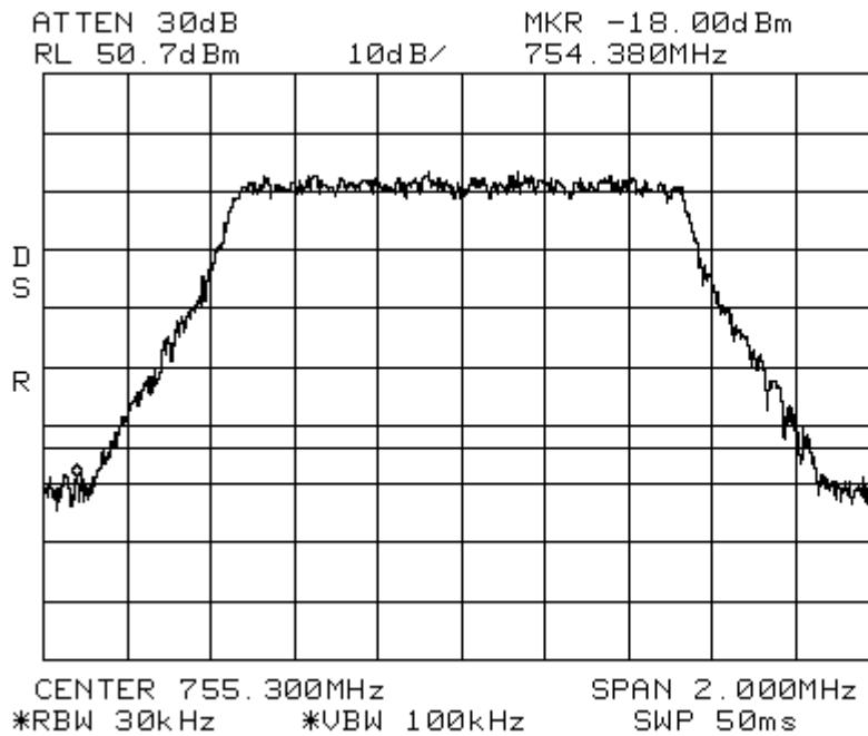
Band\_Edge LTE 3 MHz Channel Bandwidth 700UpperC 40W
