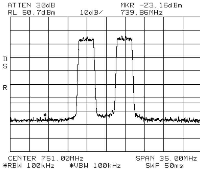
Intermodulation LTE 3 MHz Channel Bandwidth \_Apart 700UpperC 40W
