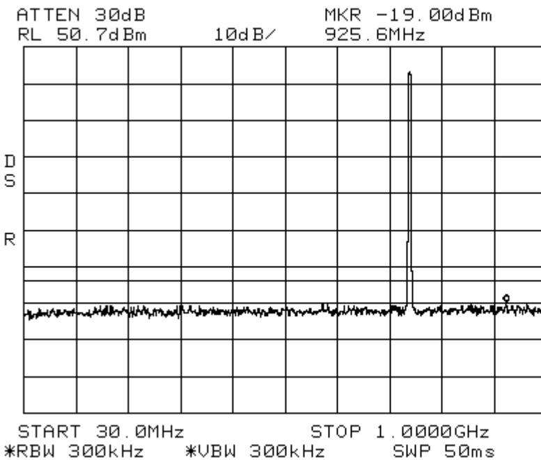
Conducted Emissions      LTE 3 MHz Channel Bandwidth      700UpperC 40W
