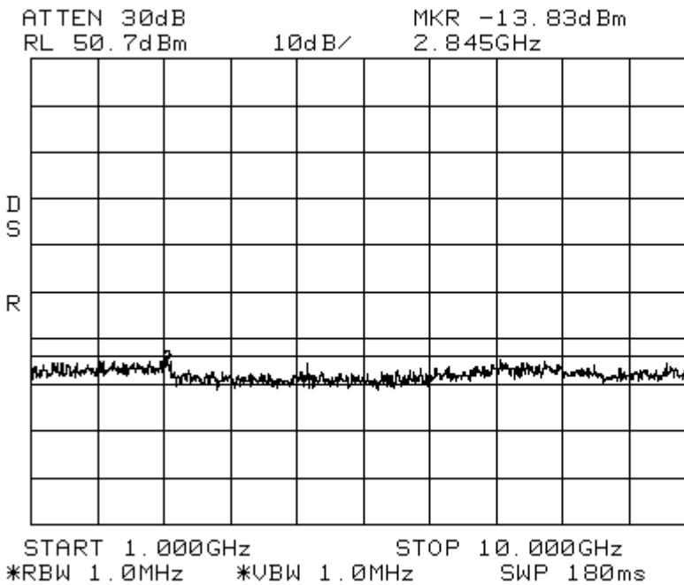
Intermodulation      LTE 1.4 MHz Channel Bandwidth \_Apart      700UpperC 40W
