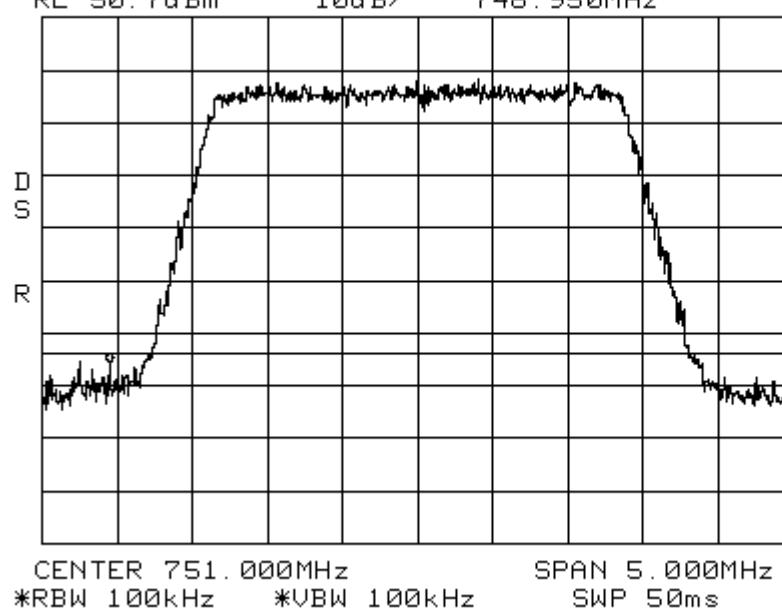
Conducted Emissions      LTE 3 MHz Channel Bandwidth      700UpperC 40W
