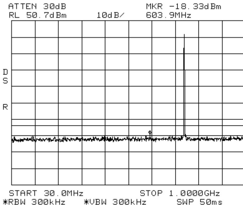
Conducted Emissions      LTE 1.4 MHz Channel Bandwidth      700UpperC 40W
