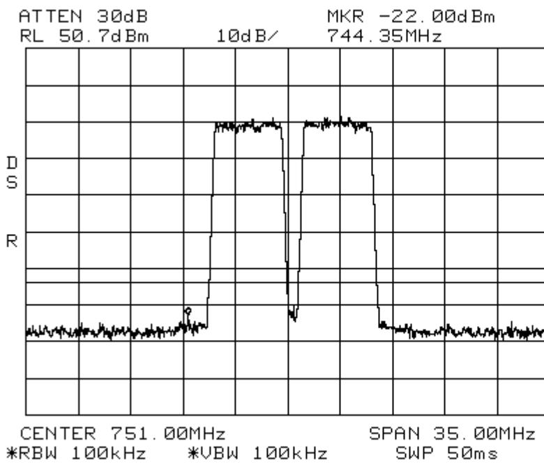
Intermodulation      LTE 5 MHz Channel Bandwidth      700UpperC 40W
