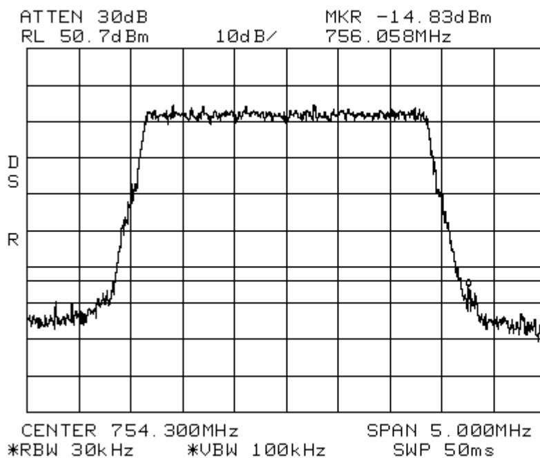
Band\_Edge LTE 5 MHz Channel Bandwidth 700UpperC 40W
