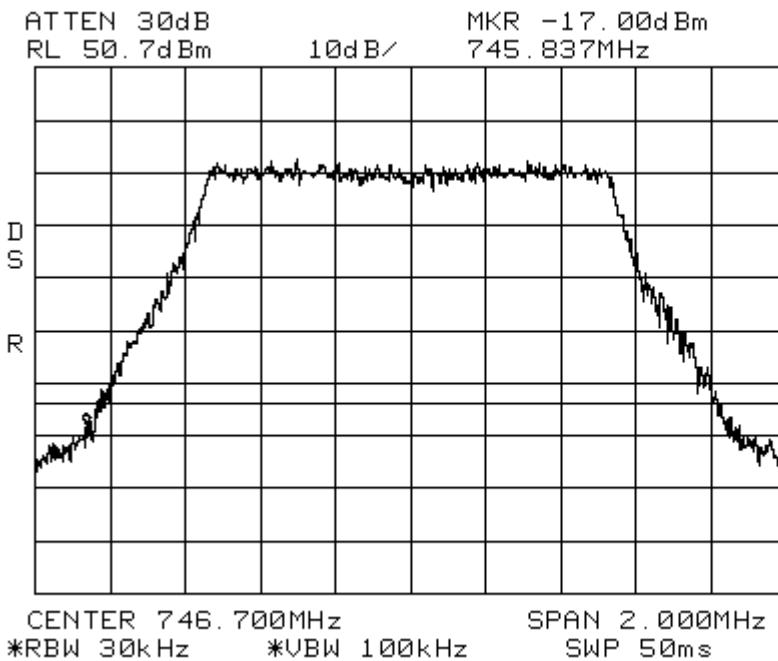
Band\_Edge            LTE 1.4 MHz Channel Bandwidth            700UpperC 40W
