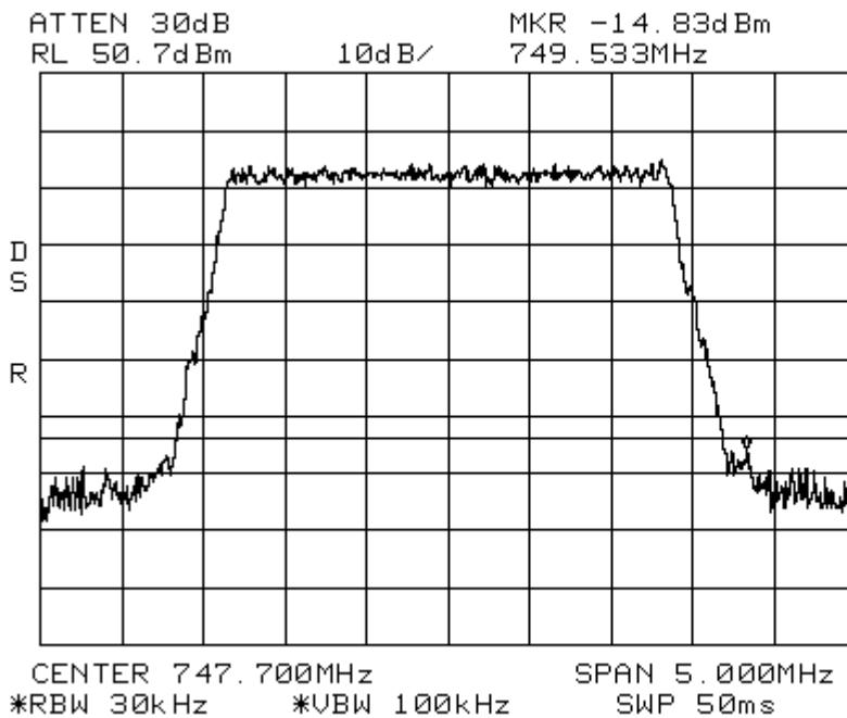
Band\_Edge LTE 3MHz Channel Bandwidth 700UpperC 40W
