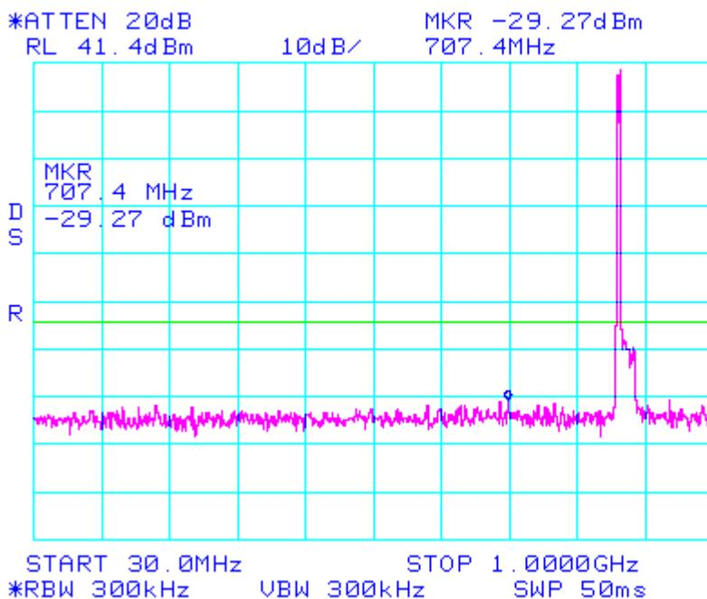
Intermodulation      GSM\_Low      CELLULAR
