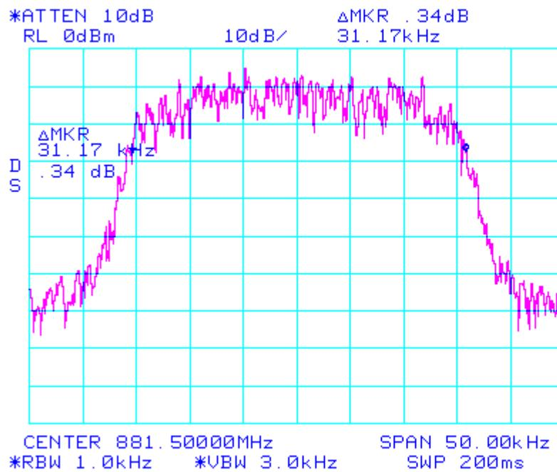
Occupied Bandwidth TDMA\_Signal\_Out
