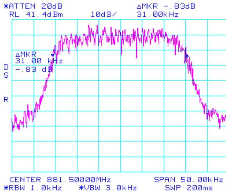
Occupied Bandwidth      GSM\_Signal\_In
