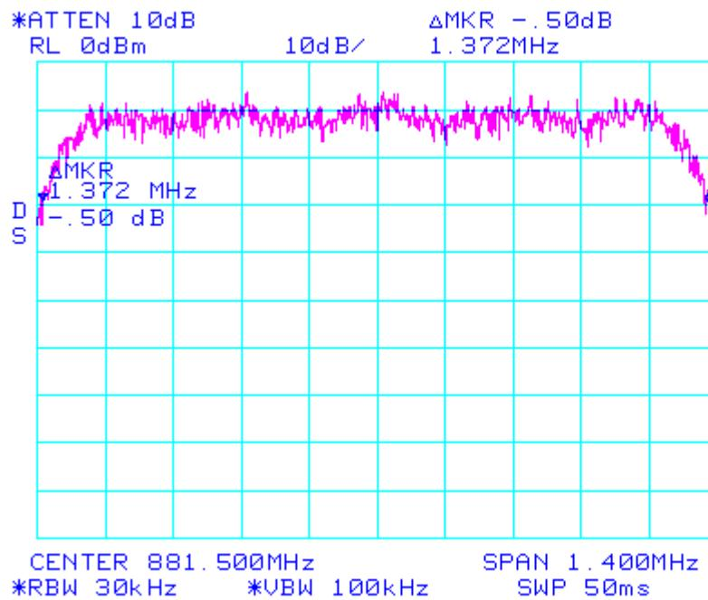
Occupied Bandwidth CDMA\_Signal\_Out
