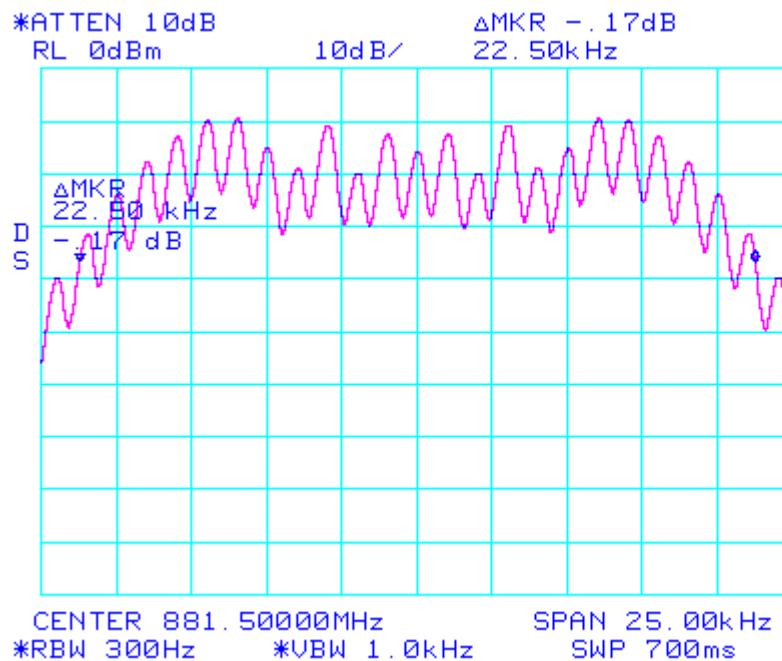
Occupied Bandwidth FM\_Signal\_Out
