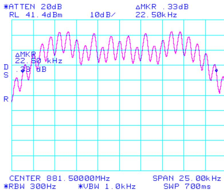
Occupied Bandwidth TDMA\_Signal\_In
