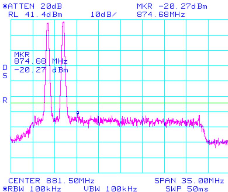
Intermodulation      GSM\_Low      CELLULAR
