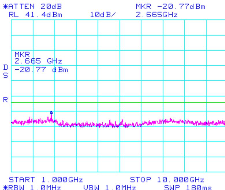
Intermodulation      GSM\_Low      CELLULAR
