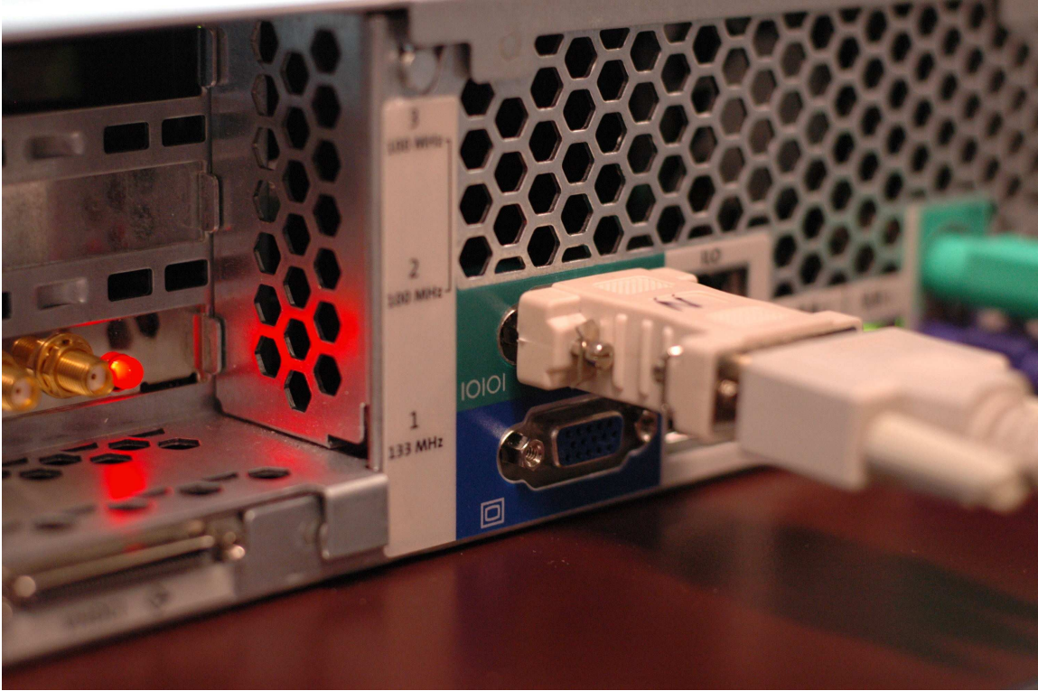
Figure 2: Close-up of a null modem cable connected to the serial console port of the HP ProLiant server.
