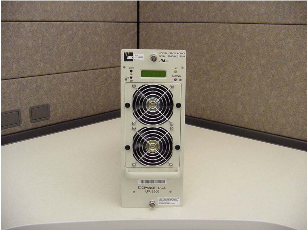
1900 MHz Linear Power Amplifier Front View
