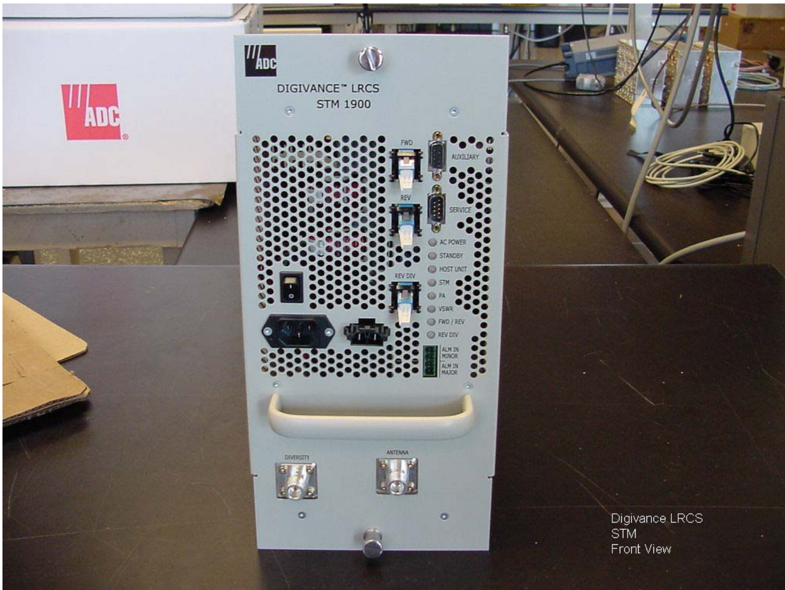
Digivance LRCS 1900 MHz Signal Transport Module - STM Front View
