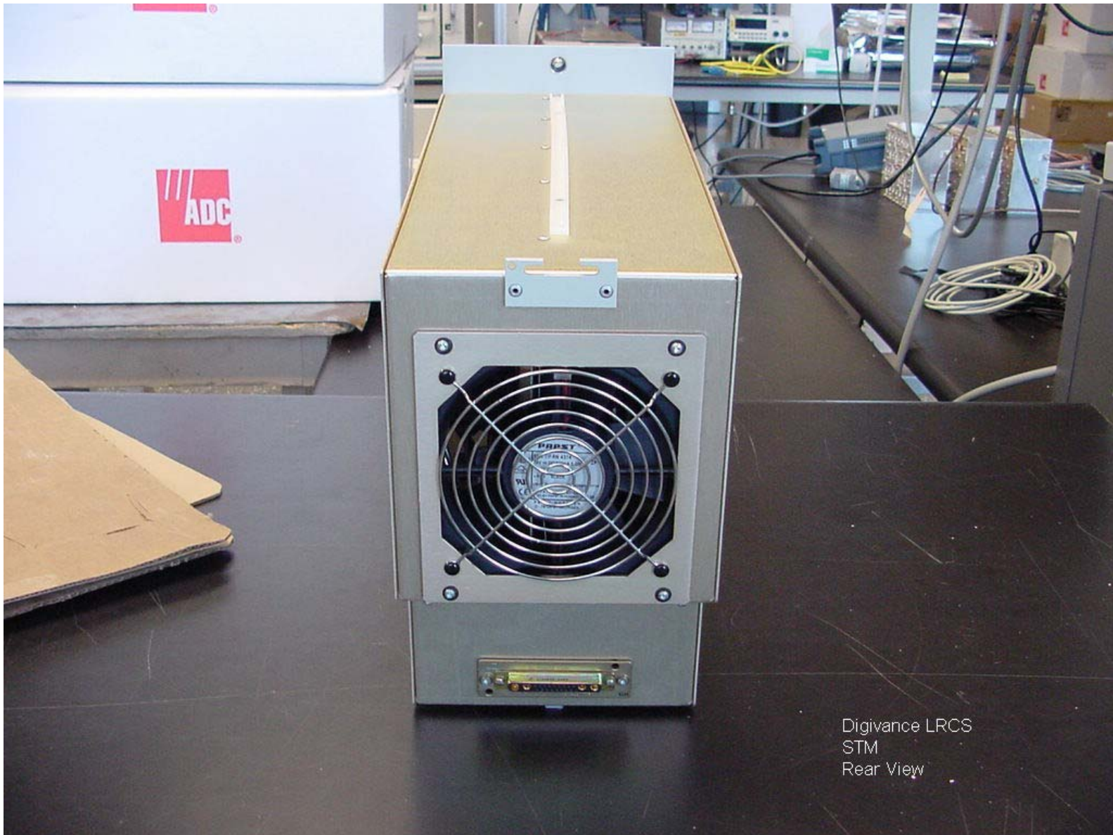
Digivance LRCS 1900 MHz Signal Transport Module - STM Rear View
