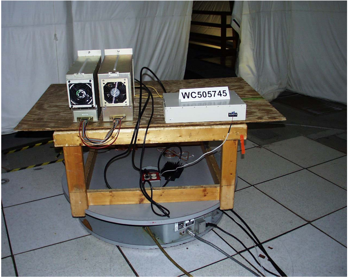
Test setup photo, radiated emissions
