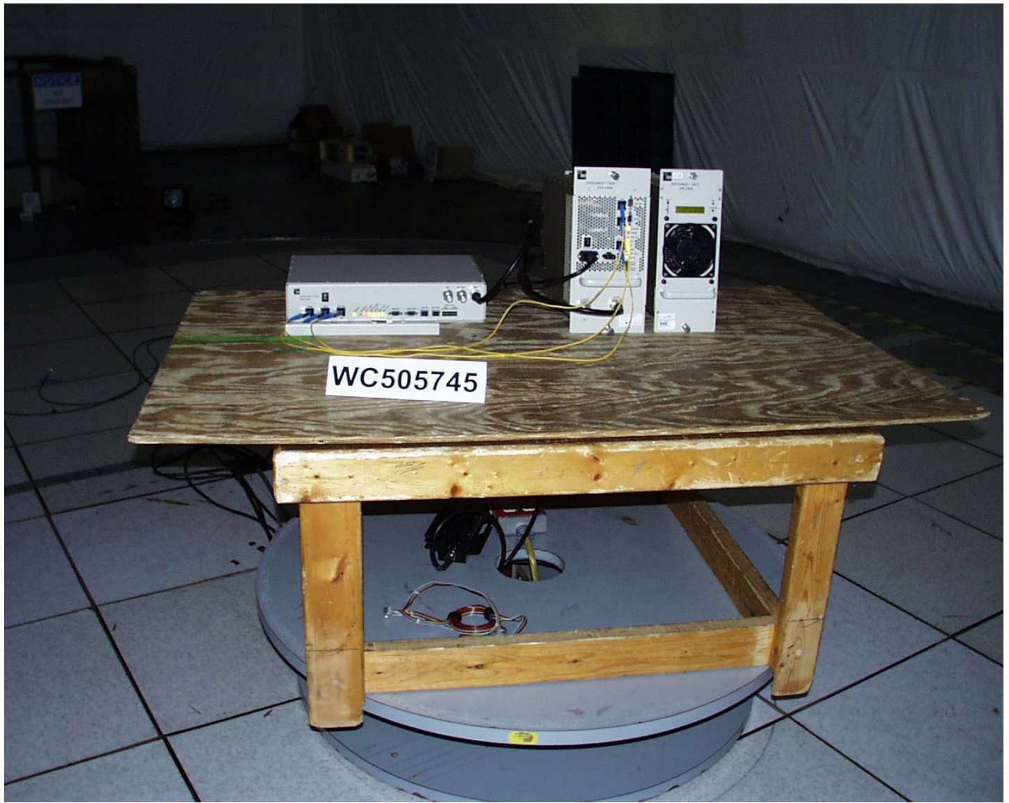
Test setup photo, radiated emissions
