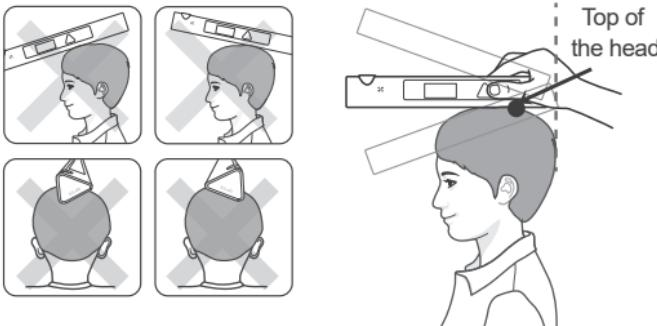
4) Press the button to take measurement. You can re-measure the height by pressing the button when you see horizontal bar on the screen.
