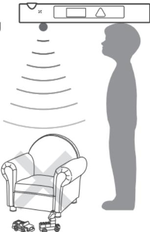
3) Place the end of the PUSH that doesn't have the ultrasonic wave sensor on the top of the head. Balance the PUSH vertically and horizontally until "PUSH" is displayed on the screen.
