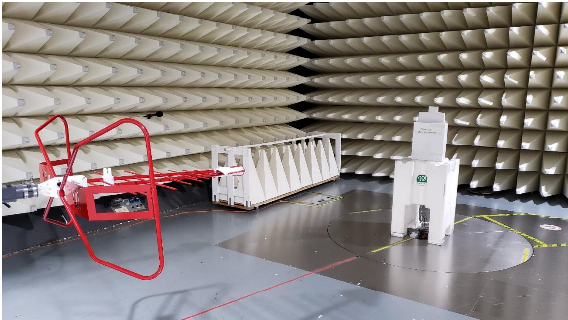
3. Radiated Emission test setup Low Range
