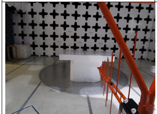
Spurious Emission Below 1GHz-Front View
