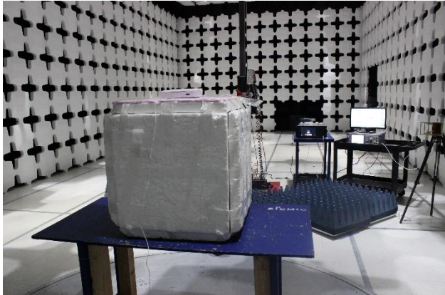
Spurious Emission Above 1GHz-Front View
