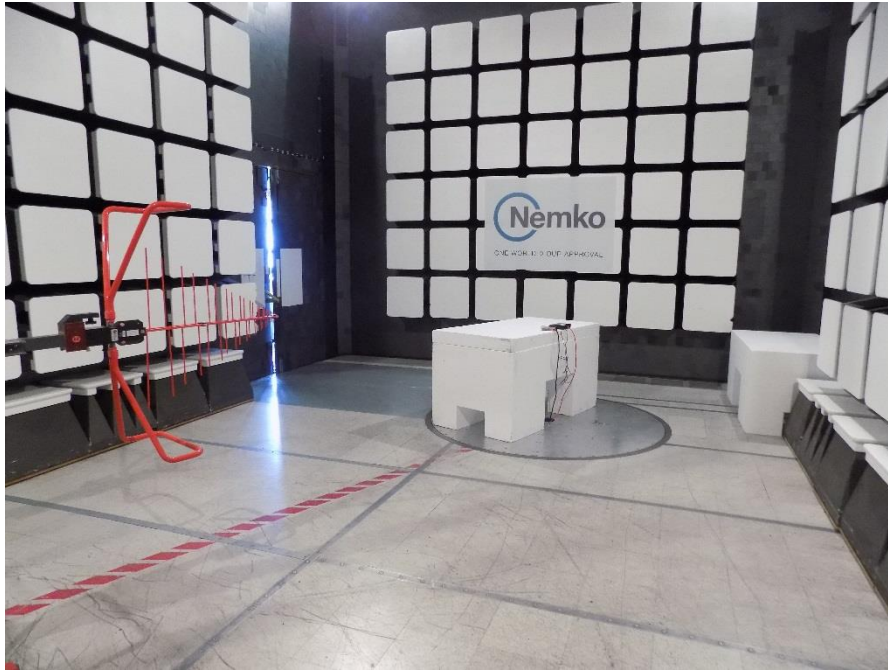
Figure 8.1-1: Radiated spurious emissions setup photo – 30 to 1000 MHz
