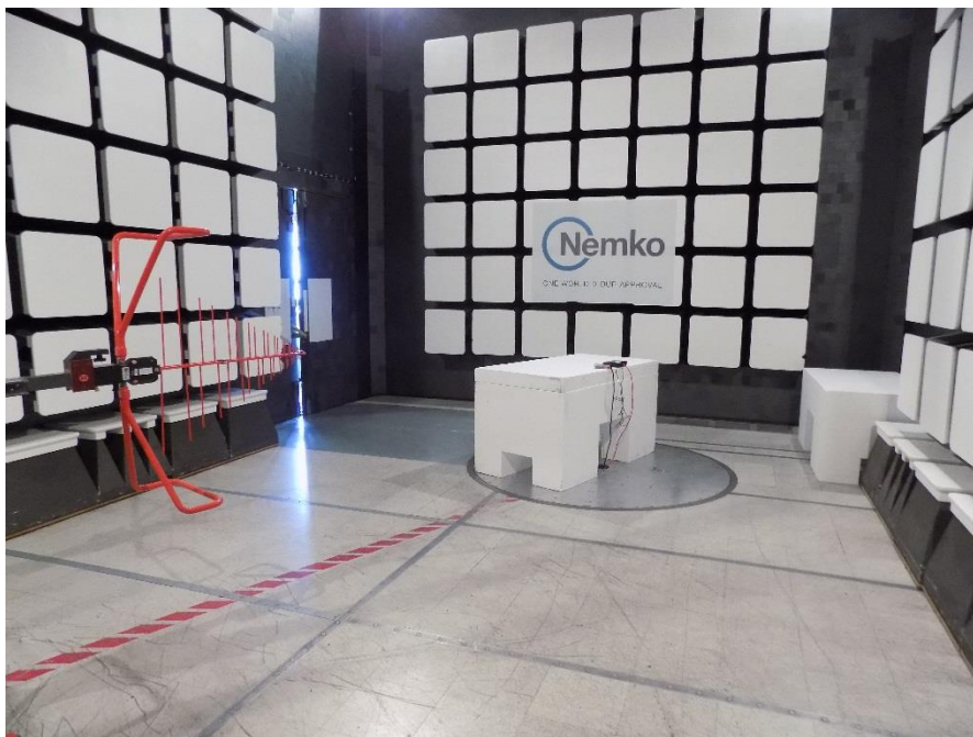
Figure 8.1-1: Radiated spurious (out-of-band) emissions setup photo – 30 to 1000 MHz
