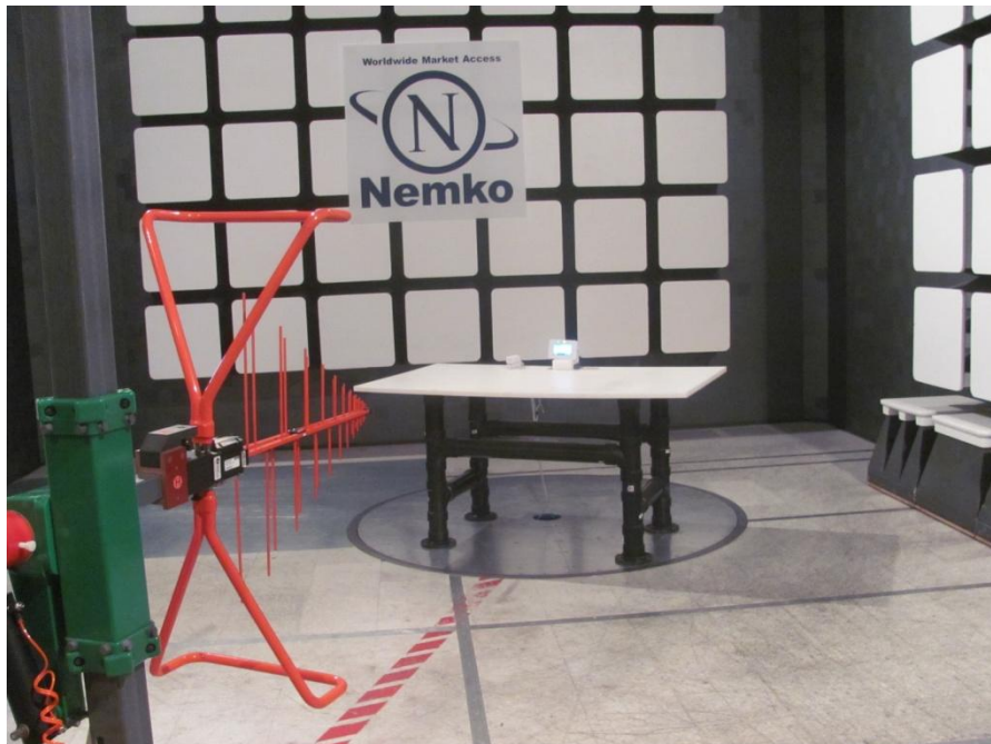
Photo 8.3-2: Field strength of emissions setup
