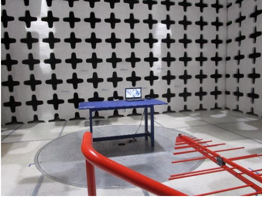
Radiated Emission Test setup (<1GHz) – Front View
