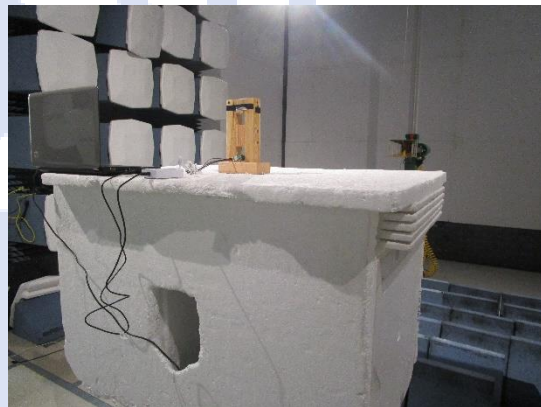
Radiated Emission Test setup (>1GHz) – Rear View
