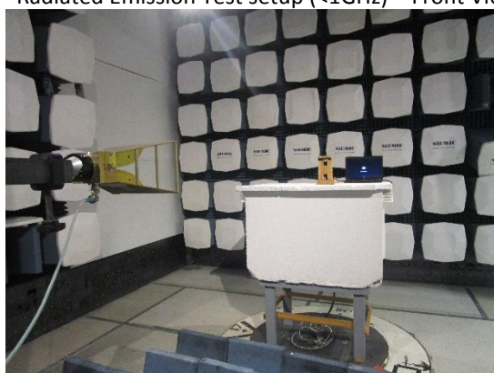
Radiated Emission Test setup (>1GHz) – Front View
