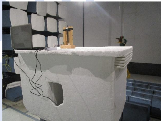
Radiated Emission Test setup (>1GHz) – Rear View
