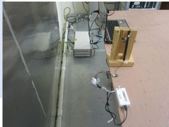
AC Line Conducted Emissions – Rear View
