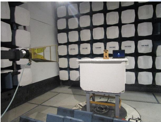
Radiated Emission Test setup (>1GHz) – Front View
