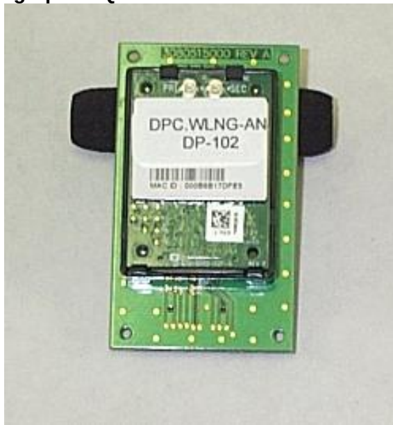
Photograph of Quatech Module Board: Top Shield removed
