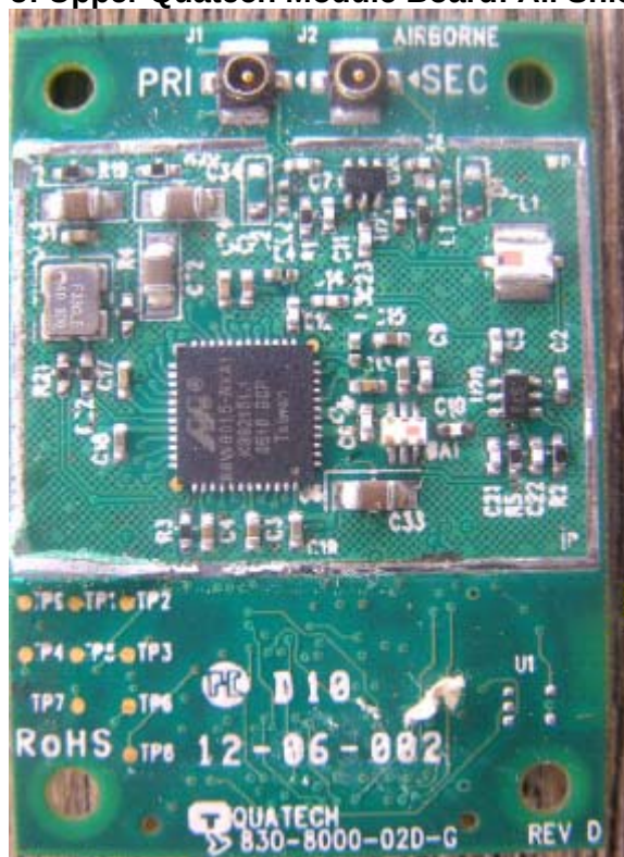
Photograph of Upper Quatech Module Board: All Shields removed
