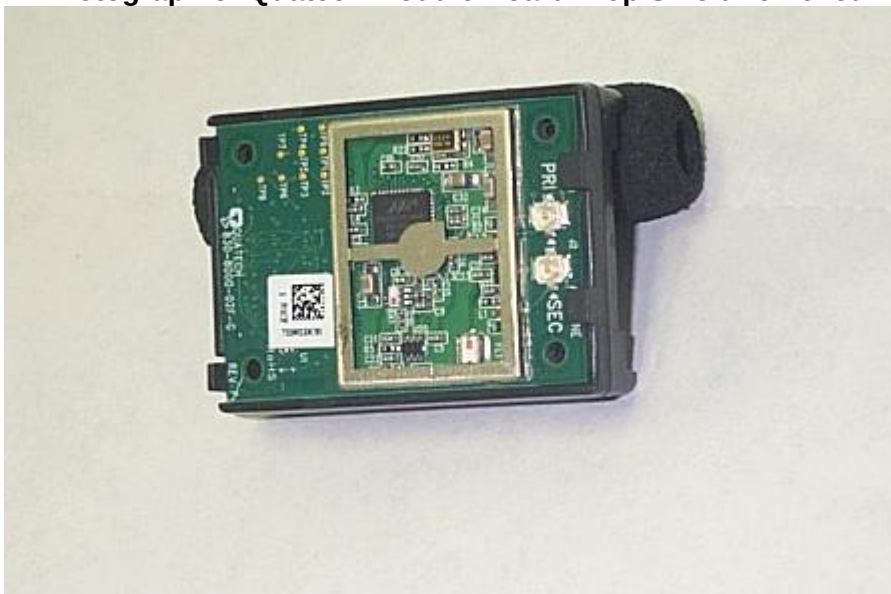
Photograph of Quatech Module Board: Top Shield removed
