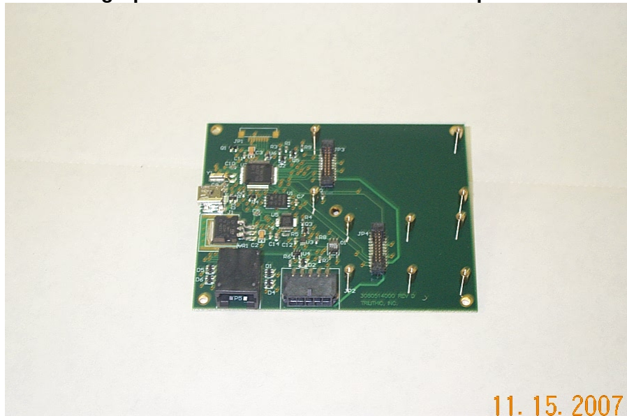
Photograph of Host Unit Mother Board: Component Side
