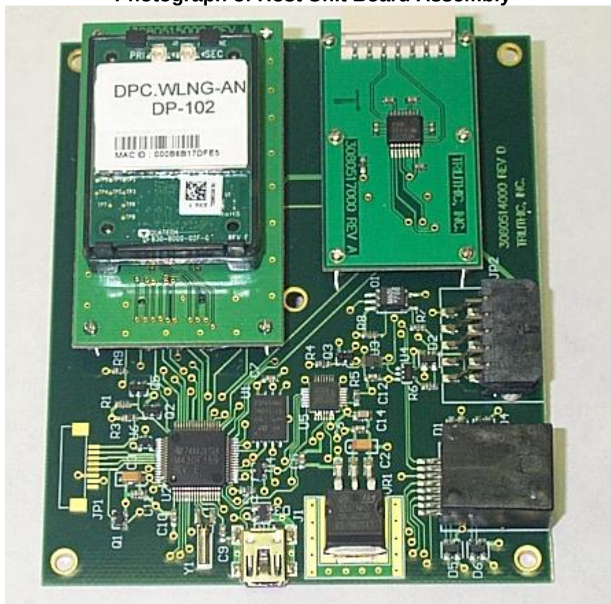
Photograph of Host Unit Board Assembly
