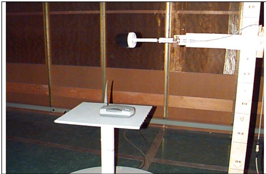
TEST SETUP: Maximum Permissible Exposure (MPE)
