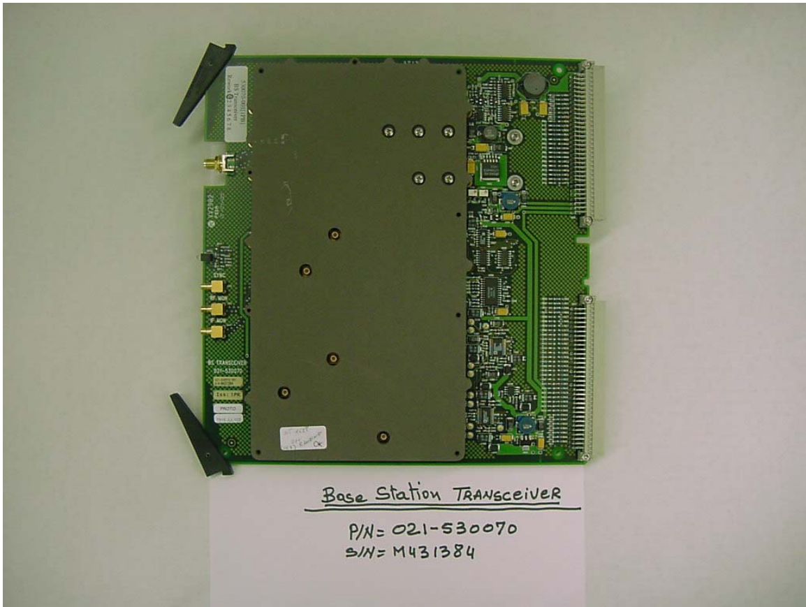
Base Station Transceiver Top
