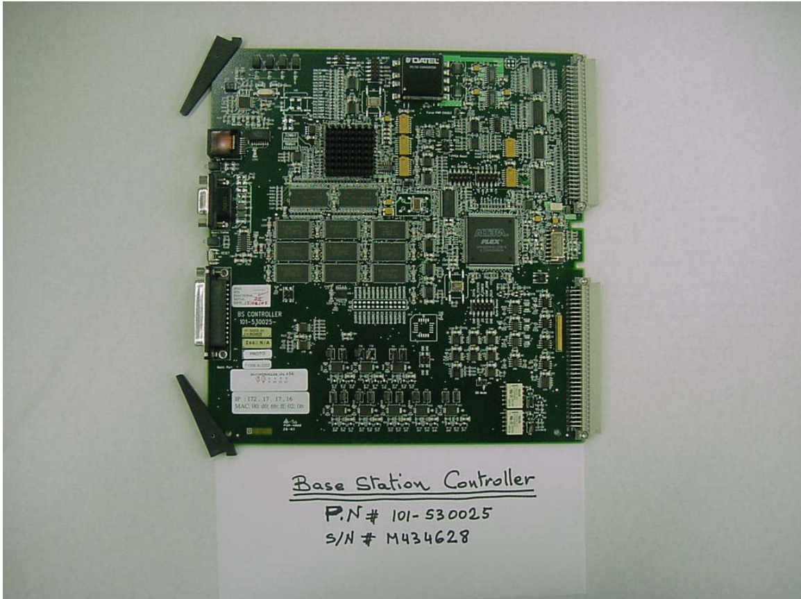
Base Station Controller Top
