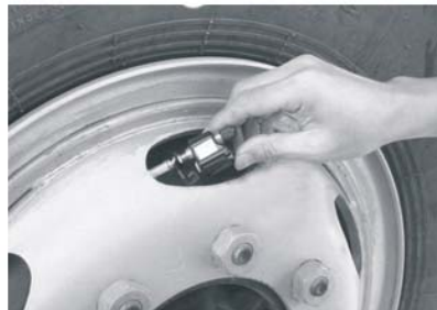
Front wheel sensor could be screwed into the valve stem directly.
