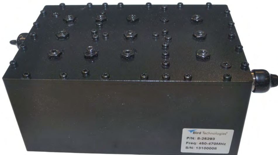
Filter Assembly side view. (part # 8-25293)
