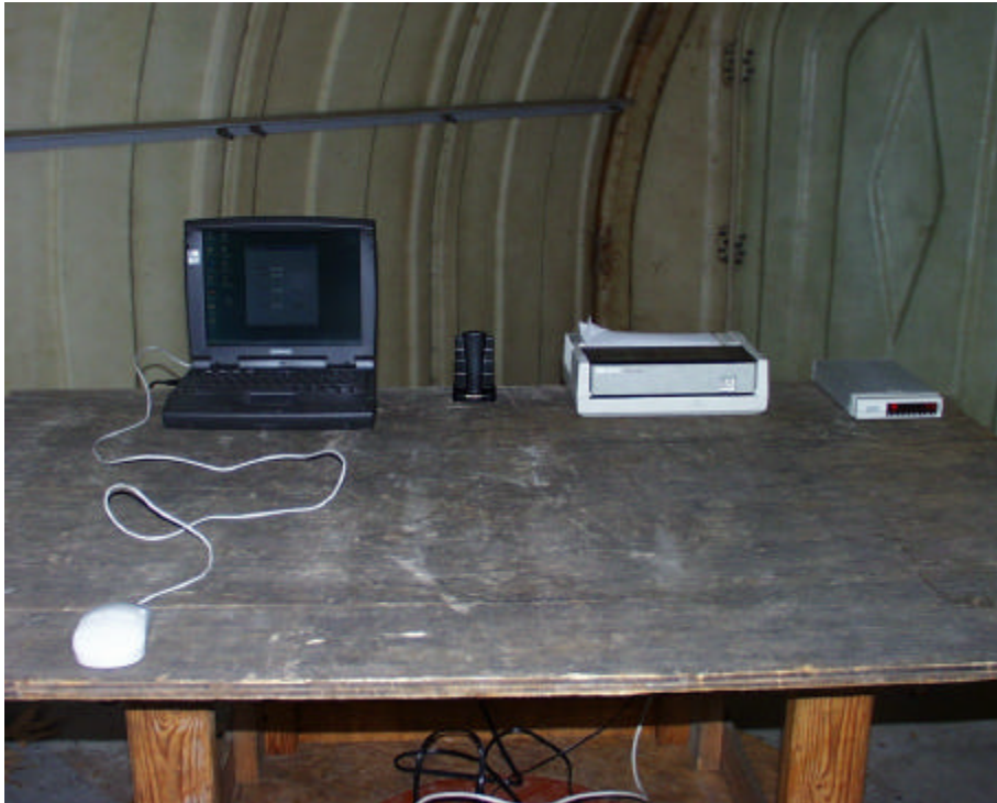
Radiated Emission below 1 GHz measurement
